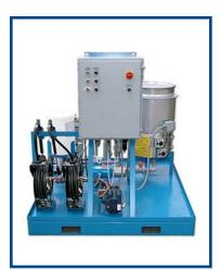
The Operator Control Panel, containing the relays, contractors and manual control switches, is built to NEMA-12 requirements and is UL listed.
